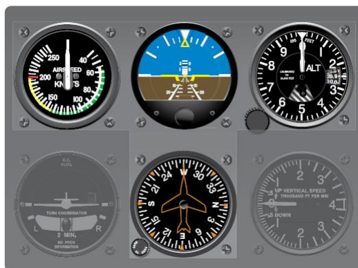
The basic T arrangement of analog flight instruments
